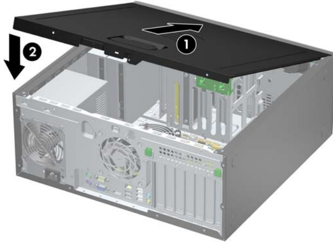
Figure 2-2 Replacing the Computer Access Panel
